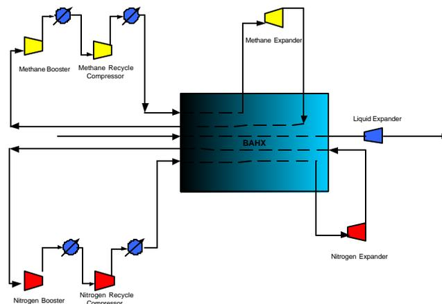
expansion the temperature of the gas descends and work is extracted from this process. The cold gas is now reintroduced to the LNG exchanger, where part of the refrigeration gained is absorbed by the gas being liquefied, and by the refrigerant gas. The warmed
