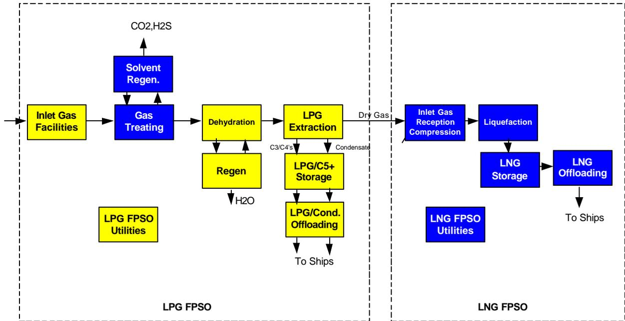
**Figure 5** Overall Project Block Diagram
